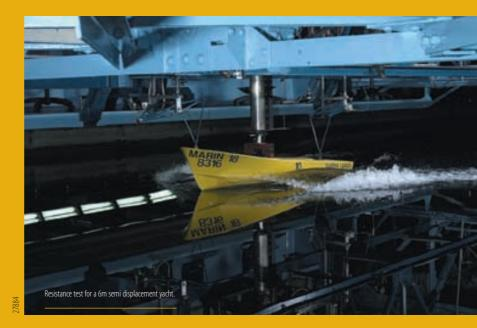
With these models it is quite easy to change a bow section or perform a keel study for a sailing yacht. Keeping the costs low, model testing becomes interesting for small yards or design offices. For a relatively small budget, model tests can be conducted and using the vast experience of MARIN, hull line
